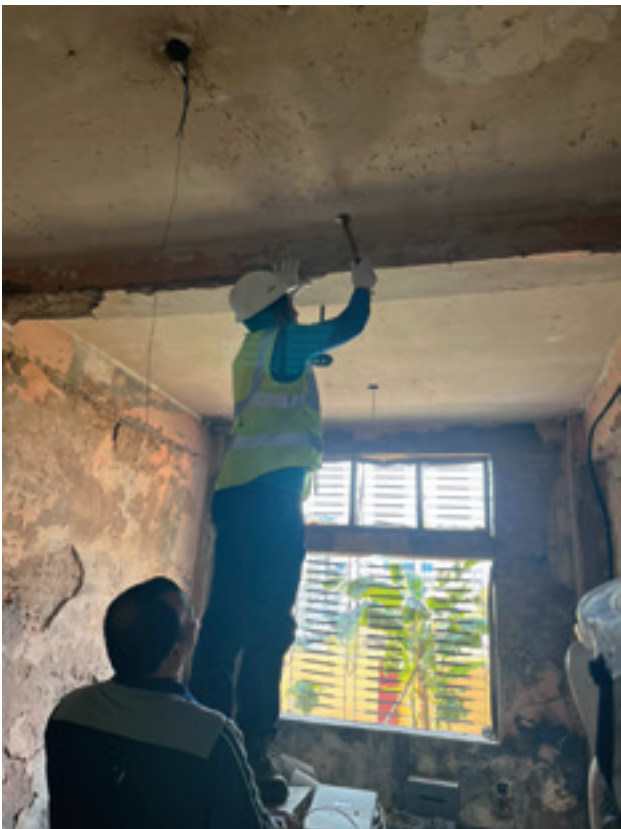
Hammer Tapping for Concrete Quality Check in the Birjunj Inland Revenue office
